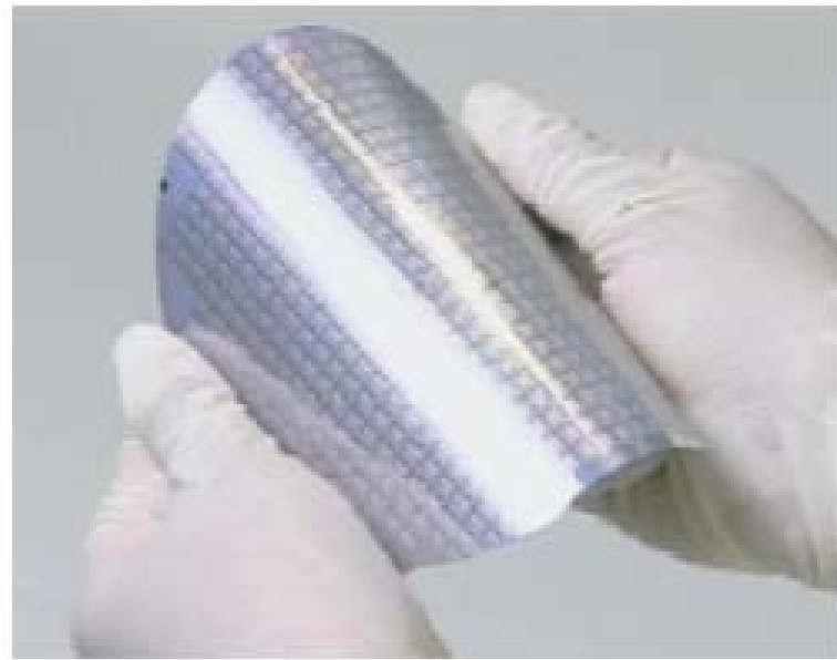
Wafer thinned to 50 microns (leti)
