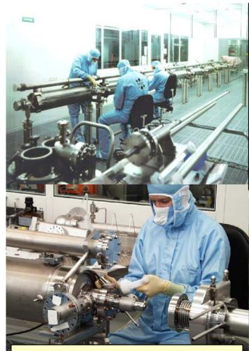
The inter-cavity connection is done in class 10 cleanroom
