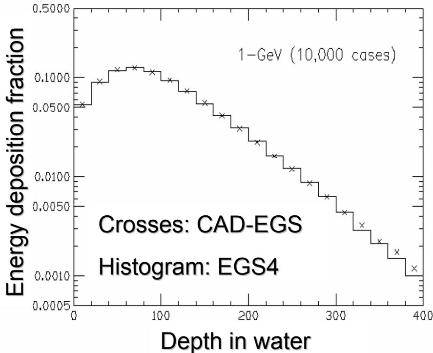
Crannel benchmark: 1 GeV electron beam in a 4 m long water cylinder, radius 12 cm, sampled in 20 segments.
