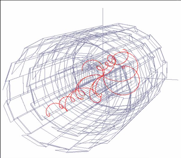
BaBar Silicon Vertex Detector as modeled by CEPack. All 320 wafers are individually represented.
