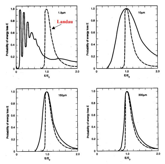
May be understood by a few, but not picked up by most simulation. Various kluges (e.g. Landau convoluted with Gaussian) help at limited thickness range and breakdown for very thin layers.
