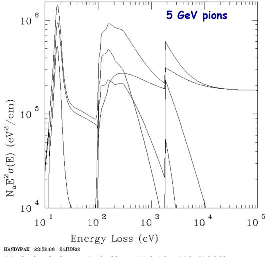
Detailed single atomic collision spectrum from a combination of atomic theory and data.
