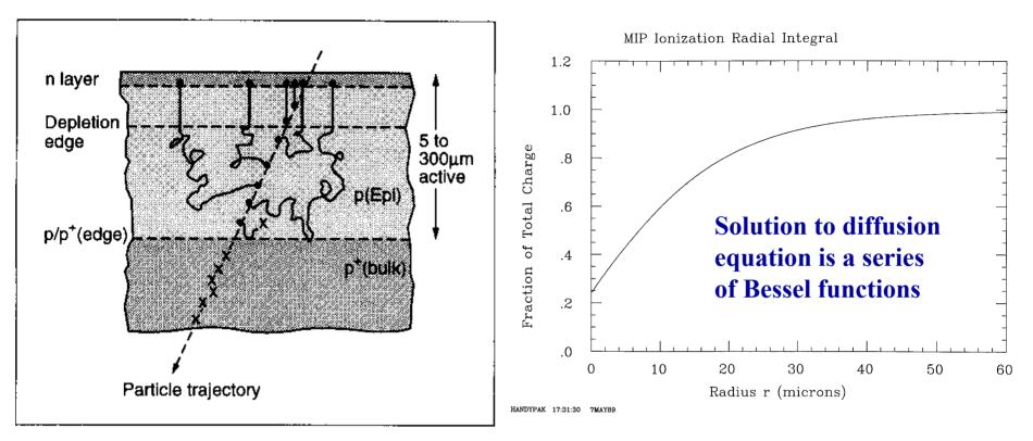
e.g. SLD VXD3 CCD has total 20 $\mu$ m EPI silicon. Only top 3-4 $\mu$ m is depleted. The diffusion in undepleted region and reflective P+ substrate are very helpful to spread out charge for better cluster centroid reconstruction.
