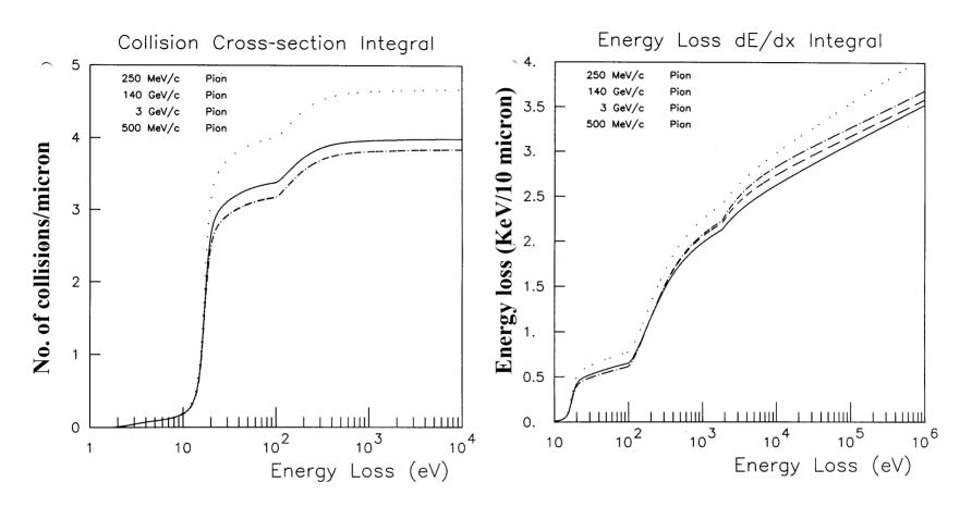
Interesting facts: ~4 collisions/micron and <1 collision/micron with E<sub>loss</sub>>100eV, but ~ half the energy loss from >1 KeV collisions in 20 micron silicon.
